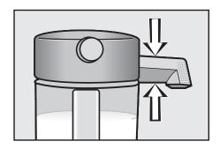
Press the spout together from the top and bottom to pull out the two pieces of the spout together. See below.
