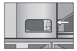
On the right side of the capsule plate is an opening. Check if a coffee capsule has jammed in there or further up in the unit.
