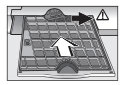
■ Push the drip tray, with the grid inserted, along the right hand side of the opening and to the back of the machine. Close the door.
