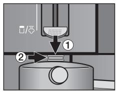
■ Press the steam lever, ①, down to connect the valve with the cappuccinatore, ②.
