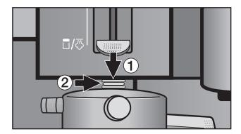
■ Press down the steam valve ① slowly and carefully to connect it to the cappuccinatore ②.
