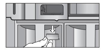
■ Pull the rubber connector downwards.
