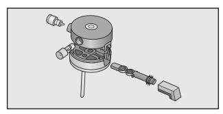
■ Reassemble the parts of the lid as shown. In order to insert the valve correctly the dot on the valve must be at the top right-hand side.
