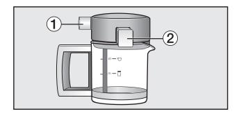
The cappucinatore must always be assembled correctly with valve ① above the handle and the spout ② at the side.
