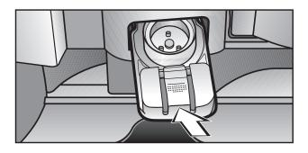
■ When prompted, remove the capsule plate and replace with the coloured descaling funnel.
