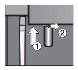
Push the froth dispenser into the machine from below, ①, and turn the cover above the spout to the right,
