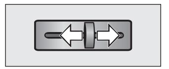
Push the slide control to the left for a finer grind or to the right for a coarser grind.
