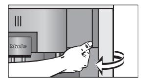
Open the appliance door by grasping the recess next to the hot water spout and pulling the door towards you.
