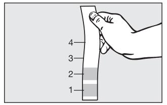
Dip the test strip in the water for 1 second and shake off any remaining water. The result is visible in about 1 minute.
