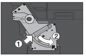
Press the light colored button on the brew unit handle, ①, and turn the handle to the right, ②.
