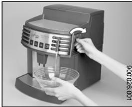
To flush out the system, place a large basin or similar container beneath the hot water outlet and turn the dial to hot water. Run off about 2 dl of water and close the valve again.
