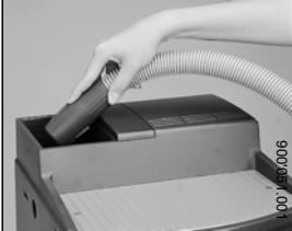
3. Using the special multifunctional tool, grasp the square end of the grinding discs spindle and slowly turn the discs in a clockwise direction until the stone or foreign body is released and can be removed. It is a good idea to use a vacuum cleaner for removing foreign bodies.
