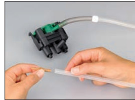
Standard: stick milk nozzle on
